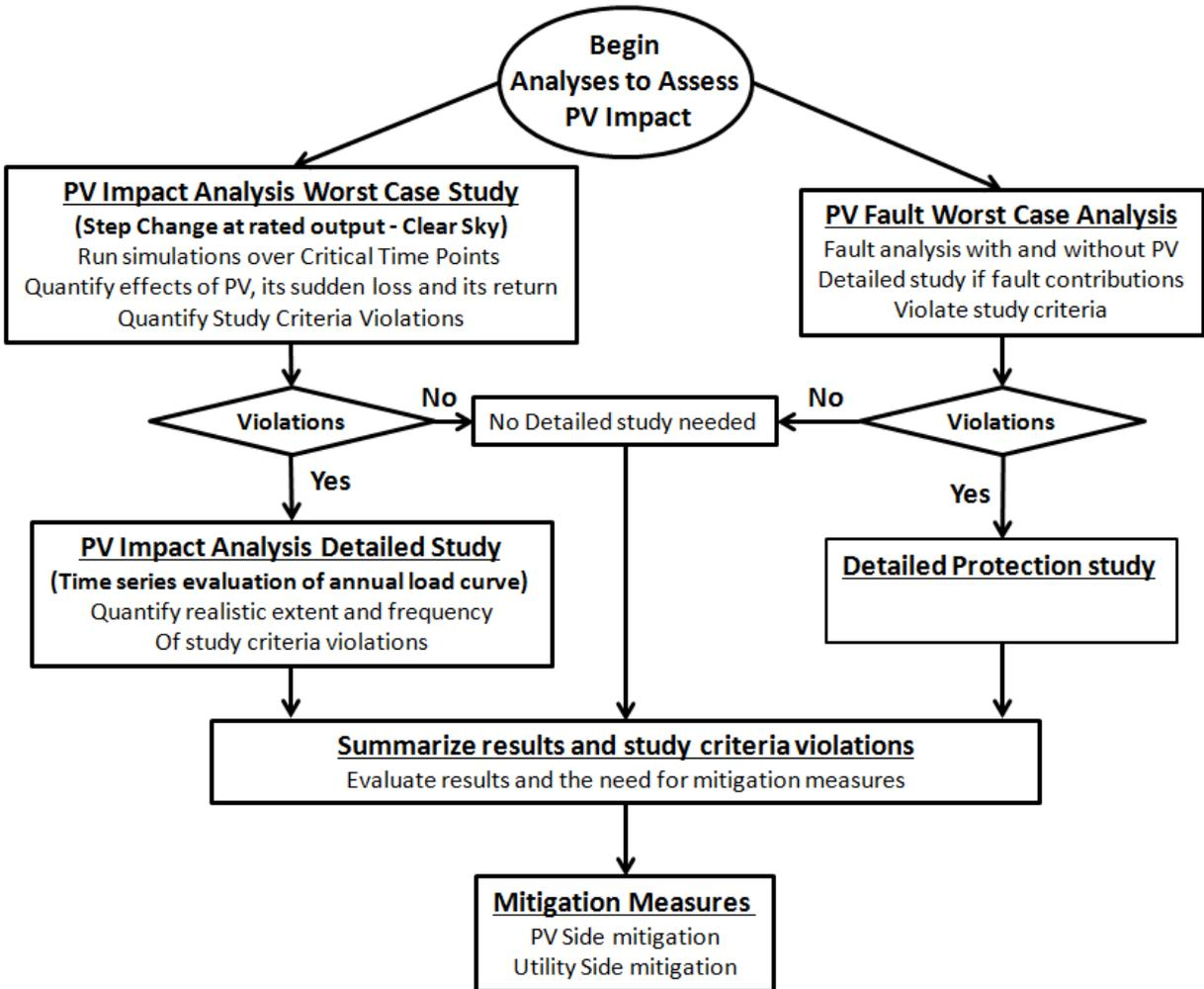
**Figure 3.2. Flowchart for performing PV impact studies**
