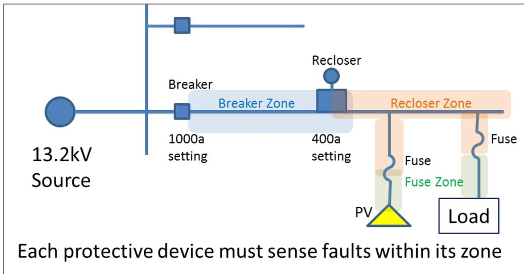
Figure 2.10. PV may desensitize protection devices to faults
