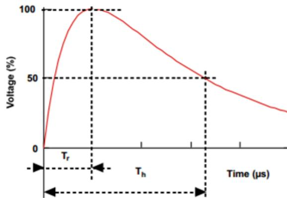
**Figure 2.6. Example of transient overvoltage**
