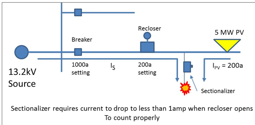
Figure 2.15. Illustration of sectionalizer miscount because of PV
