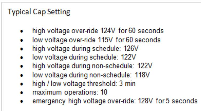
**Figure 3.6. Representative capacitor bank control and timing parameters**
