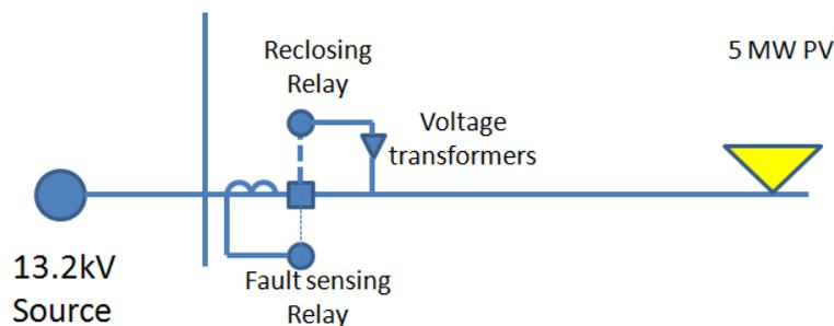
The PV must disconnect prior to the first reclosing
