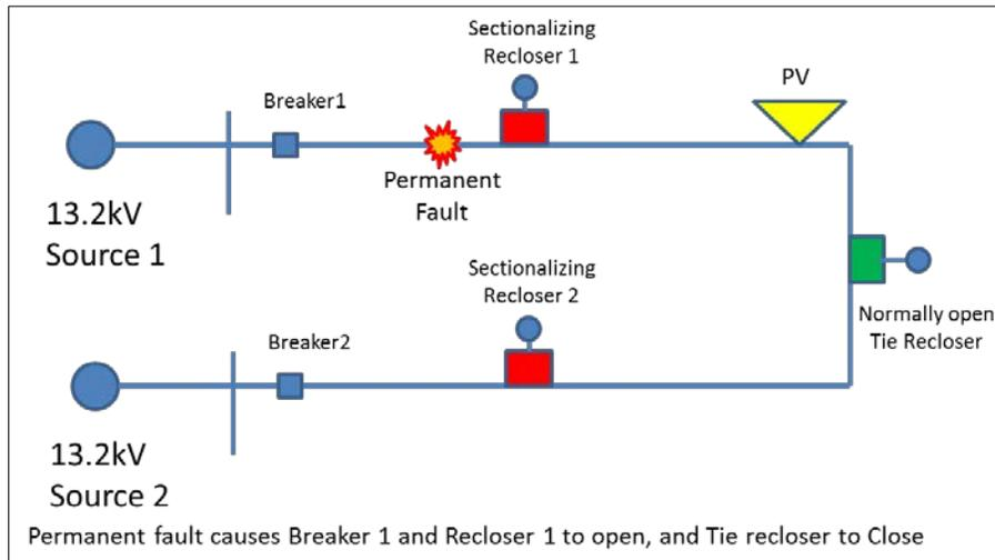
**Figure 2.19. Reconfiguration in the presence of PV**
