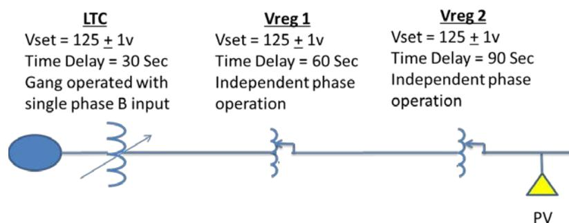
**Figure 3.4. Example of voltage regulators and control details**
