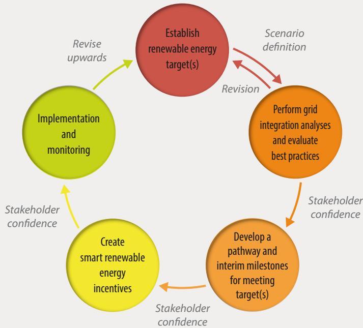
An iterative process for target-setting, analysis, and implementation helps power system stakeholders set and meet progressively higher renewable energy targets.
